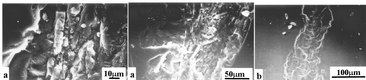
Figure 1 Scratch photograph of Ag/ \text{Al}_2\text{O}_3 samples (a) Unimplanted and (b) 1 \times 10^{17} \text{ N}^+ \cdot \text{cm}^{-2} .
